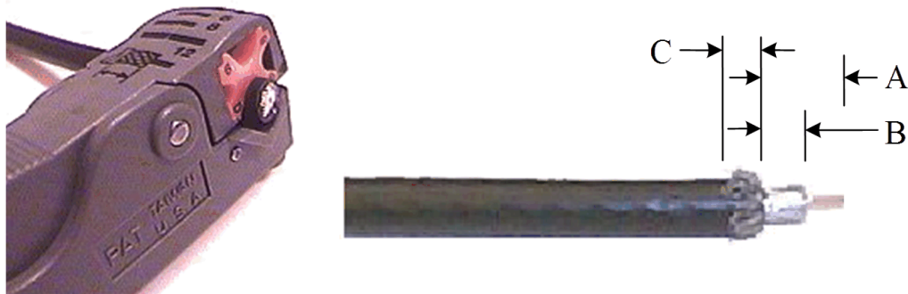
Figure B-2. Cutting Technique for Removing Foil in the Braid
